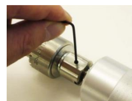
Turn screw by attached L wrench
